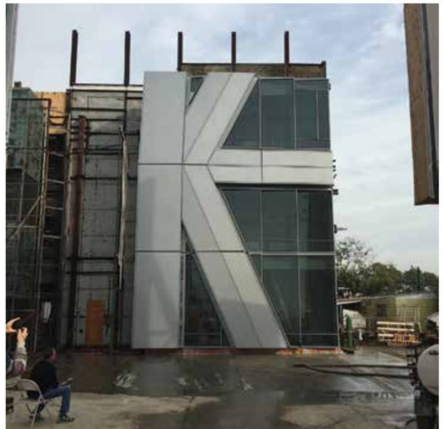
Figure 6. The façade system was racked to high levels of drift and proven to remain weather-tight.
